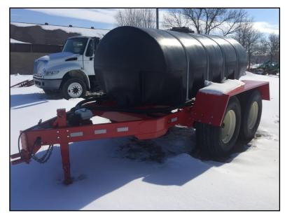
Although the trailer currently being considered is one foot wider (9° 6") than is what is legally allowed on Vermont roads (8° 6"), according to the Vermont DMV it is exempt from State permits.
