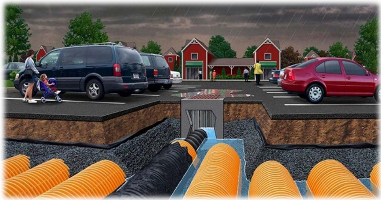
Figure 2: Illustration of chambers installed under a parking lot. Installation under the park in Bristol would be similar.
