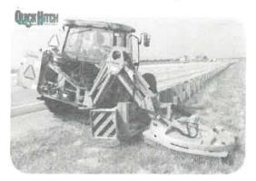
Gearbox: 540 or 1000 rpm Cutting Width: 58" Hitch: Cat. 2 & 3, Clevis Type Lower Hitch Deck Thickness: 10 Gauge Minimum Cutting Height: 2" \$20,040 Cutting Capacity: 2" Diameter
