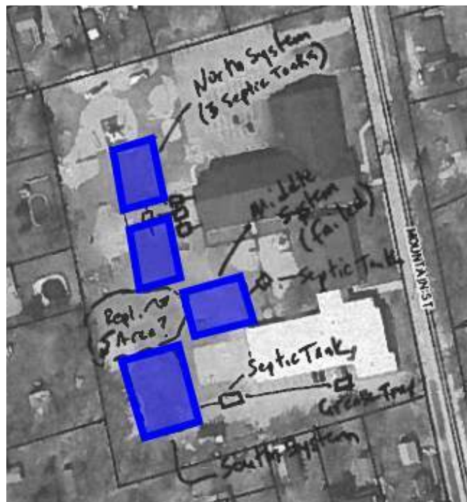
Estimated Leach Fields at Bristol Elementary School, provided by Green Mountain Engineering
