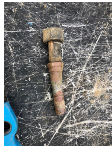
Worn Through Coupling from Above
