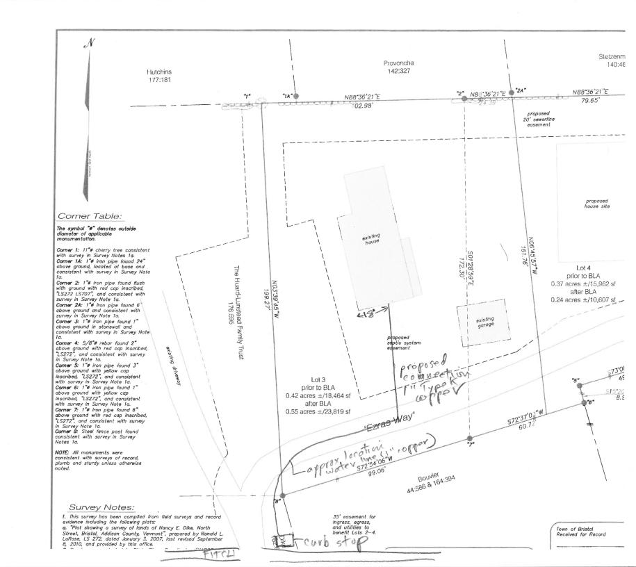
Attached Plan is proposal for water connection to new construction at 29 Ezras Way. Curb stop is at junction of Ezras Way and Fitch Avenue. Water line runs along and under Ezras Way. Connection will be made to 29 Ezras Way using 1" Type K copper water line, as specified in state permit #WW-9-1123-1. All work shall be in accordance with the approved wastewater plan and the Bristol Water Ordinance. Any existing non-compliant work shall be replaced.
