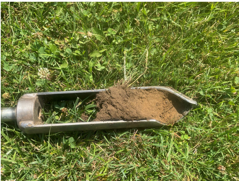
Photo F. Soil core from the central Study Area showing roadside fill and road gravel deposits.
