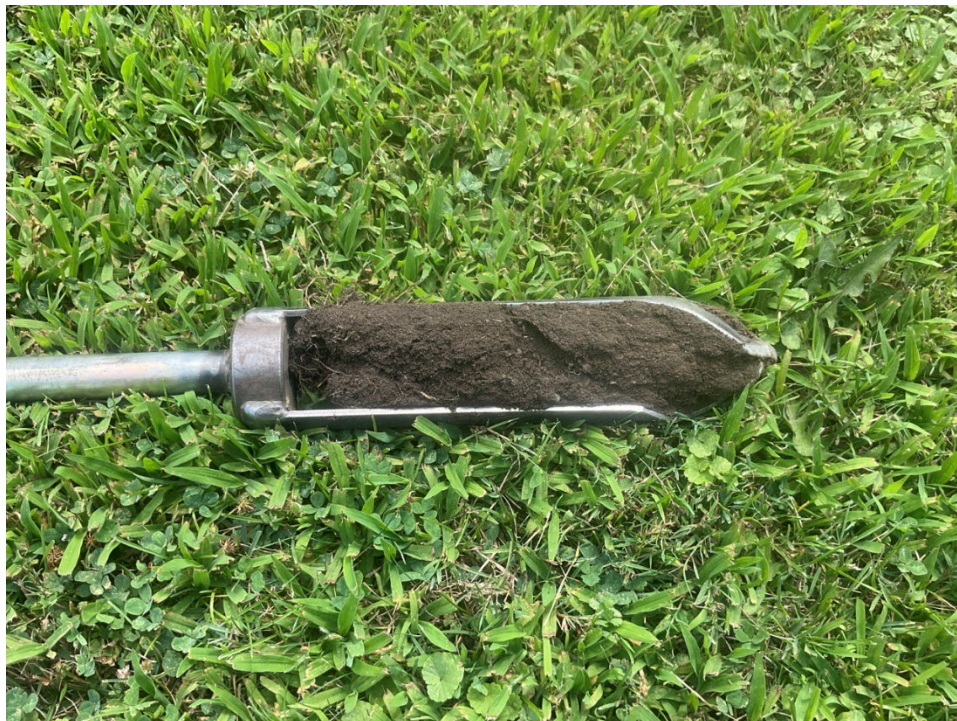
Photo K. Soil core from the western Study Area showing roadside fills.
