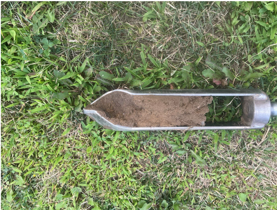
Photo E. Soil core from the eastern Study Area showing roadside fills.
