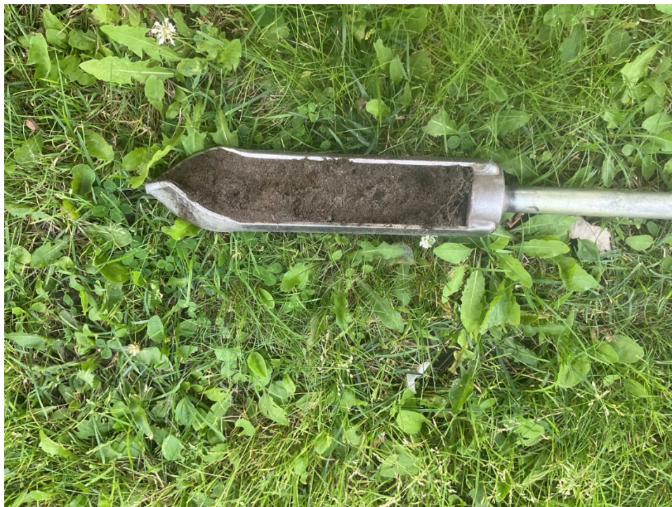
Photo M. Soil core from the western study area showing roadside fills.
